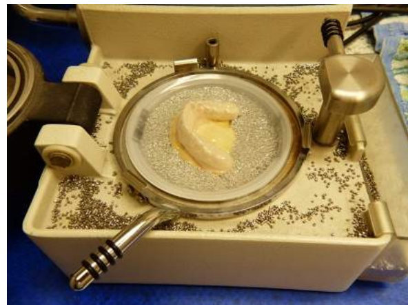
Figure 2: Bonding of the plaster model and the EVA (ethylene-vinyl acetate) sheet
